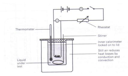
The specific heat capacity of a liquid is  $c_l$  and inner colorimeter is  $c_c$
