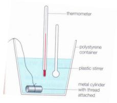
This is the most common practical used to find the specific heat capacities of solids and liquids. We usually add a hot solid (or a hot liquid) of known temperature to a cold liquid and determine the final temperature. We assume that all the heat from the hot substance goes to the cooler one if we can reduce heat loss by using insulation.
